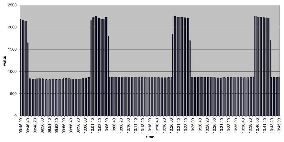
**Energy Use.** CED Designline Model HBM3, 3/1 Gn Dry Heat Bain Marie (rod element type). **Assumptions**: 1 hour measured, Quartz Halogen Gantry Lamps Half On. **Test Equipment** - Qualistar CA 8335 ( av. 884.15 w )
