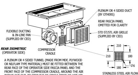
INTAKE CUT-OUT, TO STOP THE RE-CIRCULATION OF HOT AIR FROM THE COMPRESSOR. SILICON SEAL AROUND EDGES TO ENSURE THERE ARE NO AIR GAPS.
