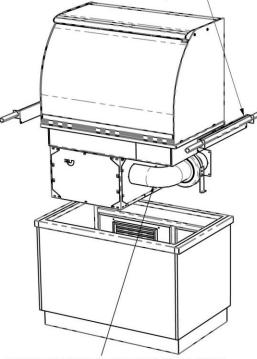
FLEXIBLE DUCTING & IN-LINE FAN SUPPLIED LOOSE. RE-ATTACH FLEXIBLE DUCTING & IN-LINE FAN TO SIDE OF COMPRESSOR CRADLE ONCE UNIT HAS BEEN DROPPED INTO PLACE. ELECTRICALY CONNECT FAN TO CONTROL BOX WITH "KETTLE PLUG"
