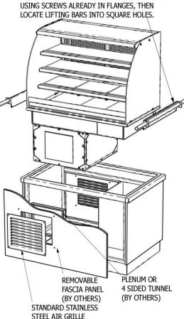
B) AIR INTAKE CUT-OUT C) AIR OUTLET CUT-OUT (CUSTOMER SIDE FASCIA PANEL)
