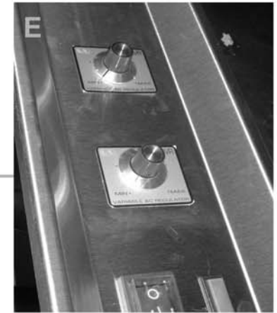
Twin Heated Gantry Rotary Controls
