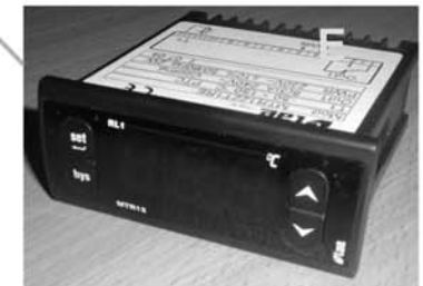
Hot Cupboard Temperature Display
